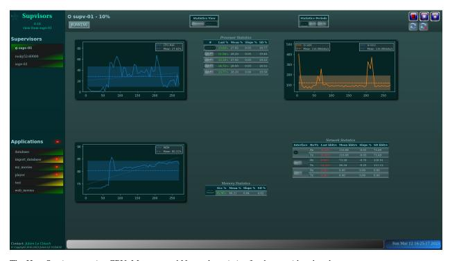
The Host Section contains CPU, Memory and Network statistics for the considered node.
